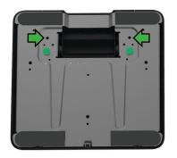
The stand supports both upright and lowered orientations. The stand is set to the lowered position from the factory. Change the orientation to upright by removing the green colored screws from the bottom of the stand and install them in the location marked by the arrows
