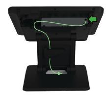
Connect the power cable to the DC power jack marked by the arrow. Then route the cable through the cable clips and through the bottom of the stand.
