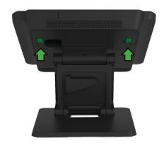
Tilt the display back to access the I/O connections and remove the cable cover.
