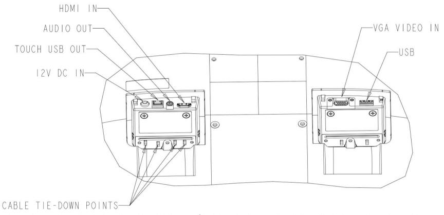
Note: Cable tie-down points can be used to tie down the cables with tie wraps. Simply loop the tie wraps through the cable tie-down points and around the cable to secure cable connections.
