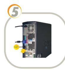
Attach USB cable from MSR device to the USB port on the rear of the computer.
