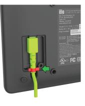
Connect the micro USB cable. Ensure the rubber gasket (red) is all the way inside the cable cover area.
