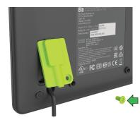
Install the cable cover by installing the top side first and rotating it down. Secure the door with the M3 screw included.
