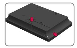
Install USB cable and route cable through the bottom of the opening as shown.
