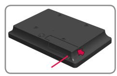
4 (Optional) The monitor can be attached to any standard 75mmx75mm VESA mounting bracket using the 4 - M4x8mm mounting screws included with the monitor.
